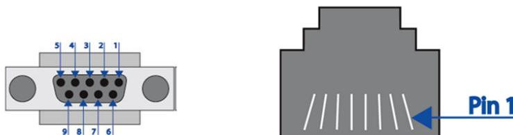
**Figure 63** DB-9 to RJ45 connector
