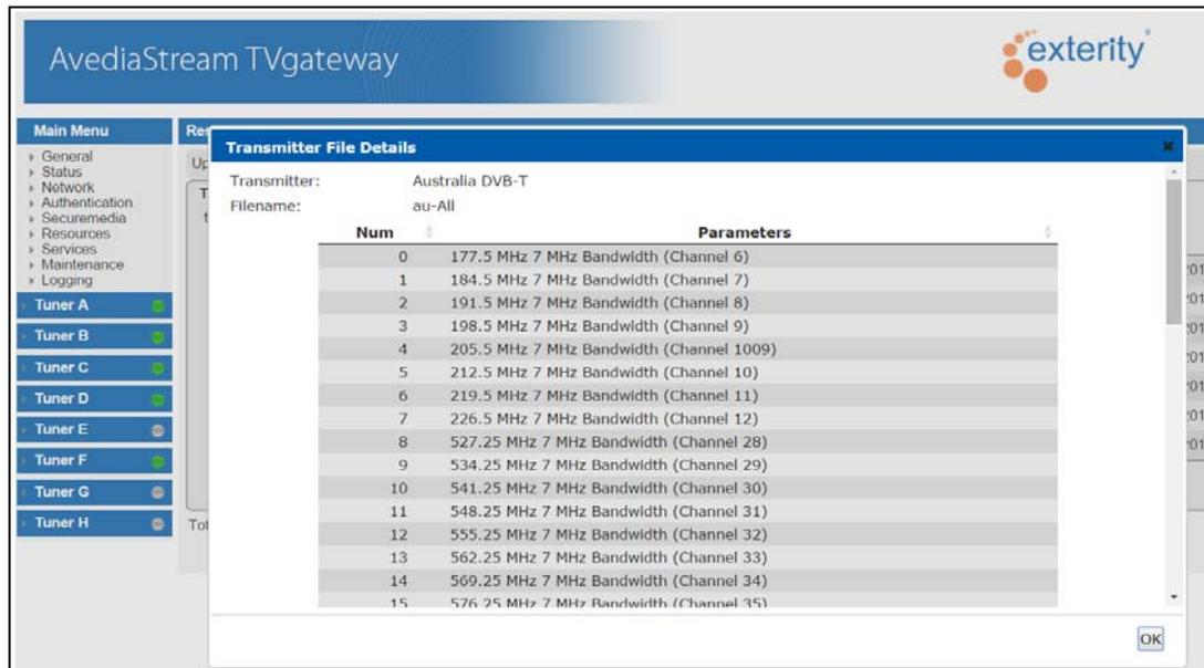
**Figure 27** Transmitter file details (AvediaStream g4448)
