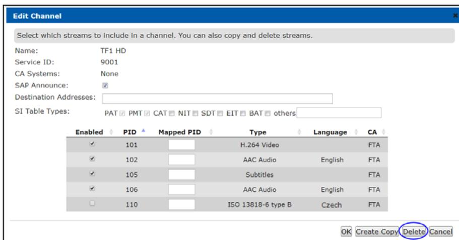
**Figure 40** Deleting duplicate channels
