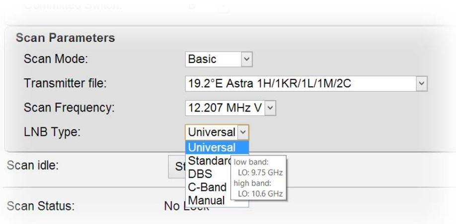
**Figure 22** Local oscillator frequency
