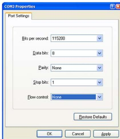
**Figure 64** Serial port settings
