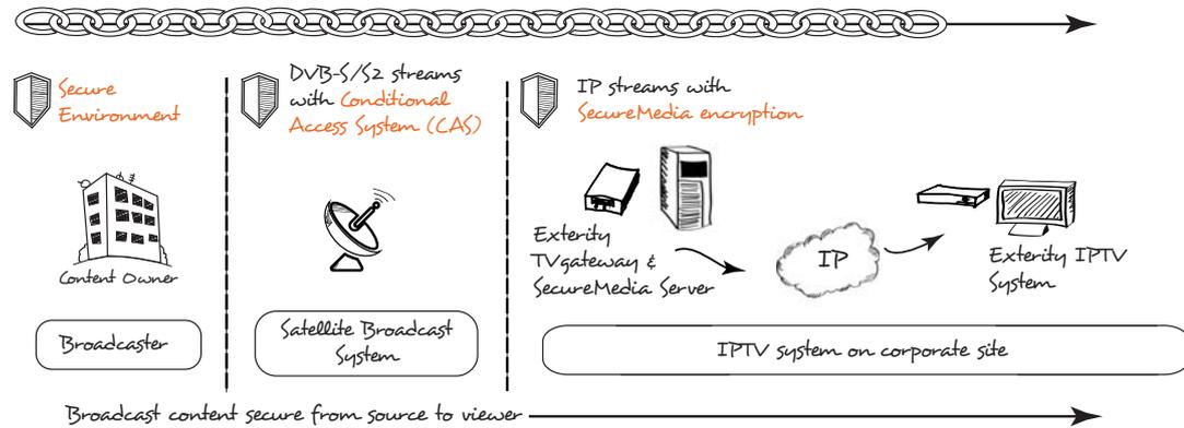
**Figure 1** Using the g4415-sm TVgateway with SecureMedia to protect video content
