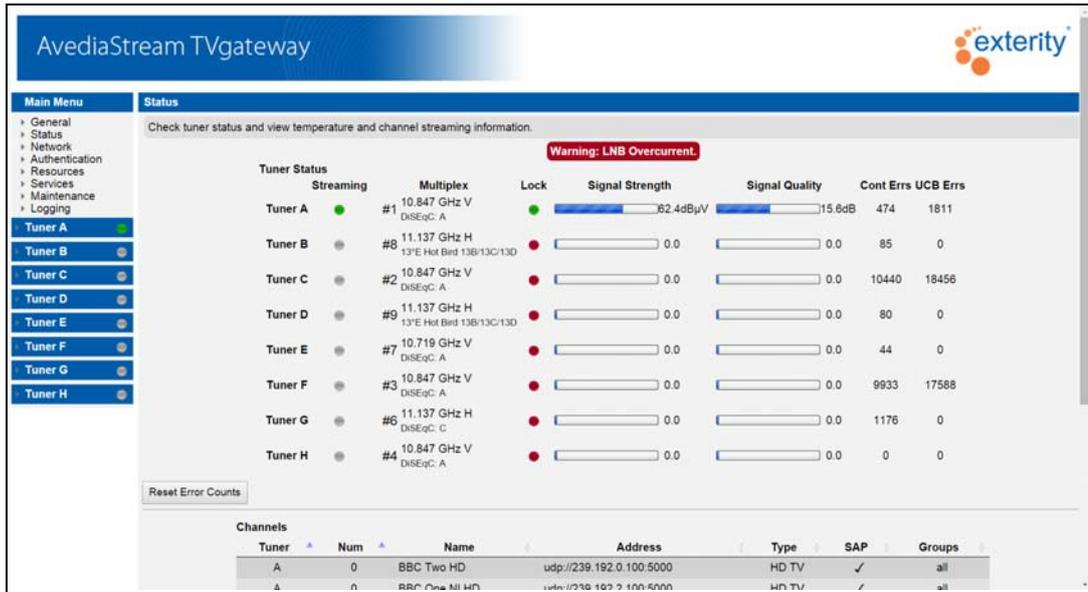
Figure 47 TVgateway Status Page with over current warning (AvediaStream g4418)
