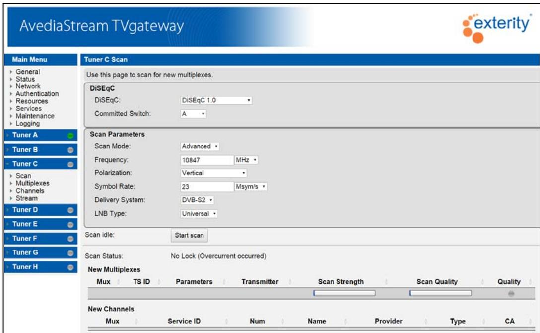
Figure 48 TVgateway Scan Page with over current warning (AvediaStream g4418)
