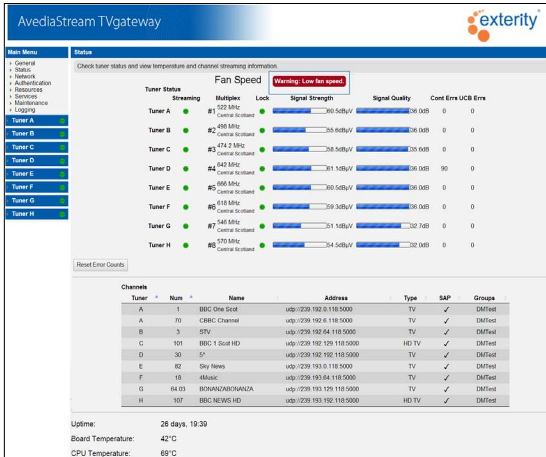
**Figure 46** TVgateway Status Page with fan speed warning (AvediaStream g4448)
