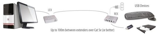
$<sup>^{\</sup>ast}$  Supports Category cabling with Cat 5e being the minimum recommended. Cat 6 and 7 are supported.
